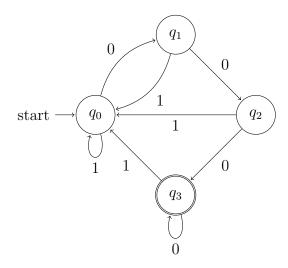
Let's think about the strings that are accepted by this DFA. If we start at the start state, how can we get to the accept state? For instance, this machine accepts the string 000. In general, this machine accepts strings that end in three zeroes. Keep in mind that this also includes those strings that end in three or more zeroes. We say that the machine accepts any string in the set  $\{w000 \mid w \in \Sigma^*\}$ , where in this case,  $\Sigma^*$  is the binary alphabet of 0 and 1.
